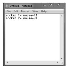
In this case, socket 1 is set to move the cursor to the Left at speed 3, whereas socket 2 moves it to Up at speed 1. Any combination of direction and speed is possible on any of the sockets.
