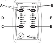
You can pair up to three wireless switches with each channel of CONTROL PRO, allowing collaboration between several users. If you attempt to pair a fourth switch, the switch that was used least recently will be replaced with the new one. The other two switches are unaffected.
